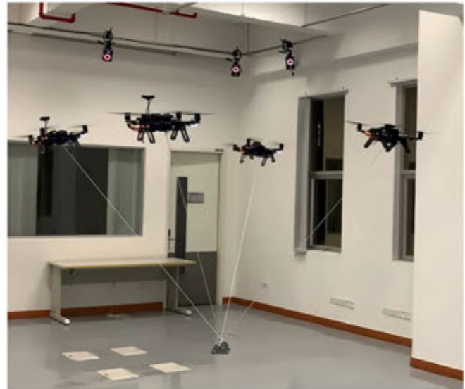
多架空中載具重型負載運輸 Load transportation by multiple aerial vehicles
